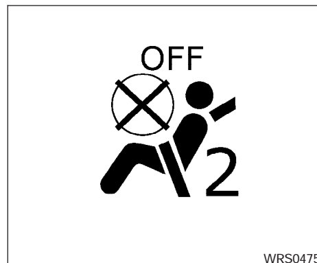
Front passenger air bag and status light
